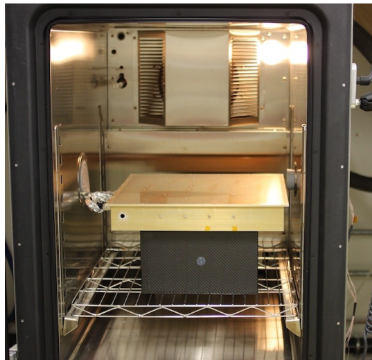
POLAR in climatic chamber: Thermal test
