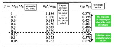
If the companion is massive enough (>5 times the WD mass), the system will never settle into RLOF accretion but the WD will plunge into the companion.
